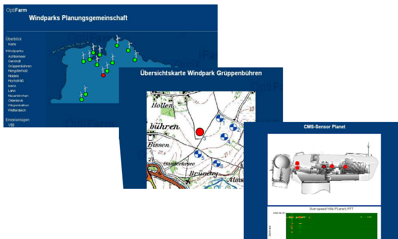
OptiFarm hierarchy from wind farm overview to alarm of the CMS sensor.
