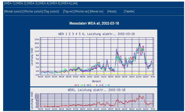
Overview of the energy produced by the various turbines in the wind farm
