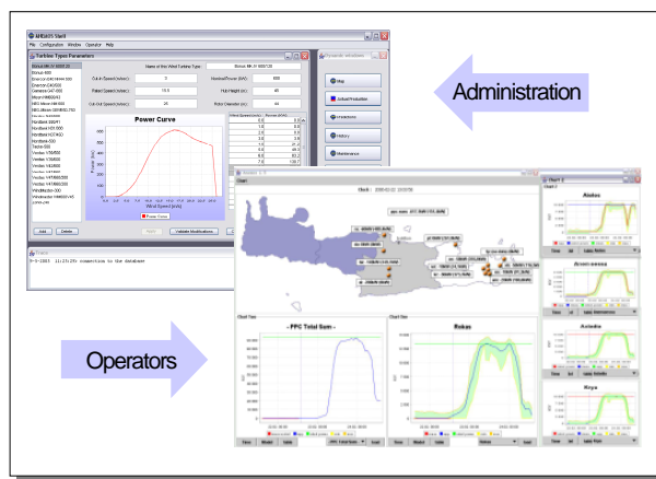
Fig. 7: Ergonomic graphical user interfaces were developed to visualise predictions and administrate the system.
